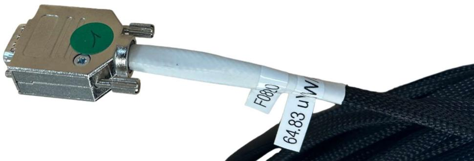
FIGURE 21 : CONNECTEUR DB9 MALE D'UNE SONDE TRANSFERT, POUR BRANCHEMENT SUR LE MODULE TRANSFERT
