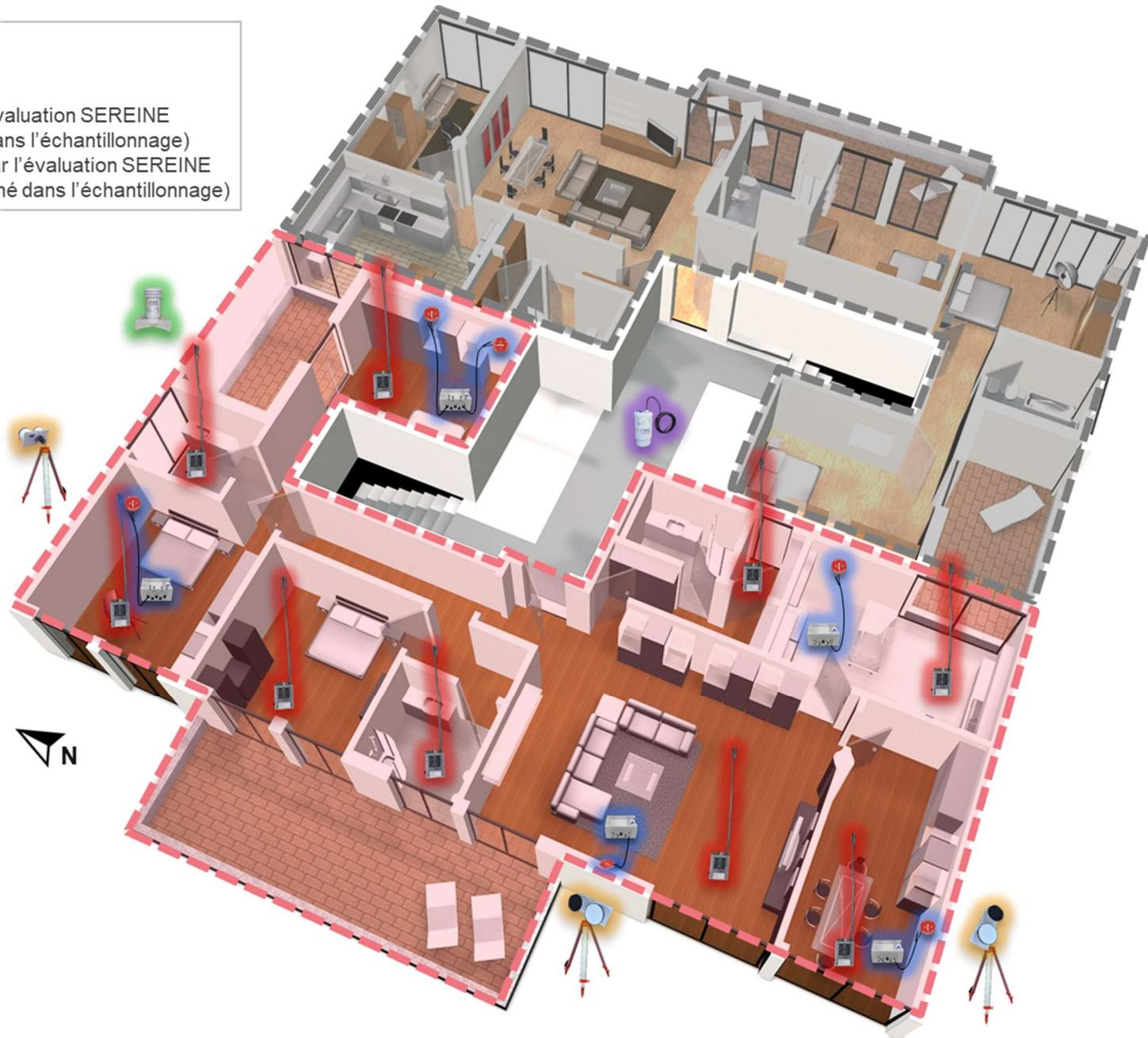
FIGURE 10 : PRINCIPE D'INSTRUMENTATION D'UNE EVALUATION SEREINE ENVELOPPE DE LOGEMENT COLLECTIF
